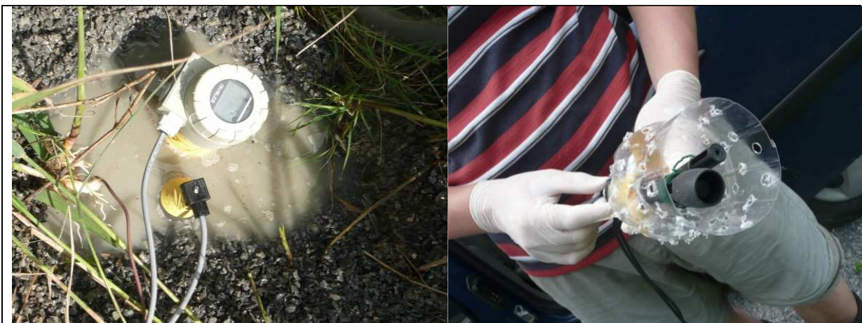
Placing of field electrodes for continual monitoring of water temperature, electrical conductivity and oxygen concentration
